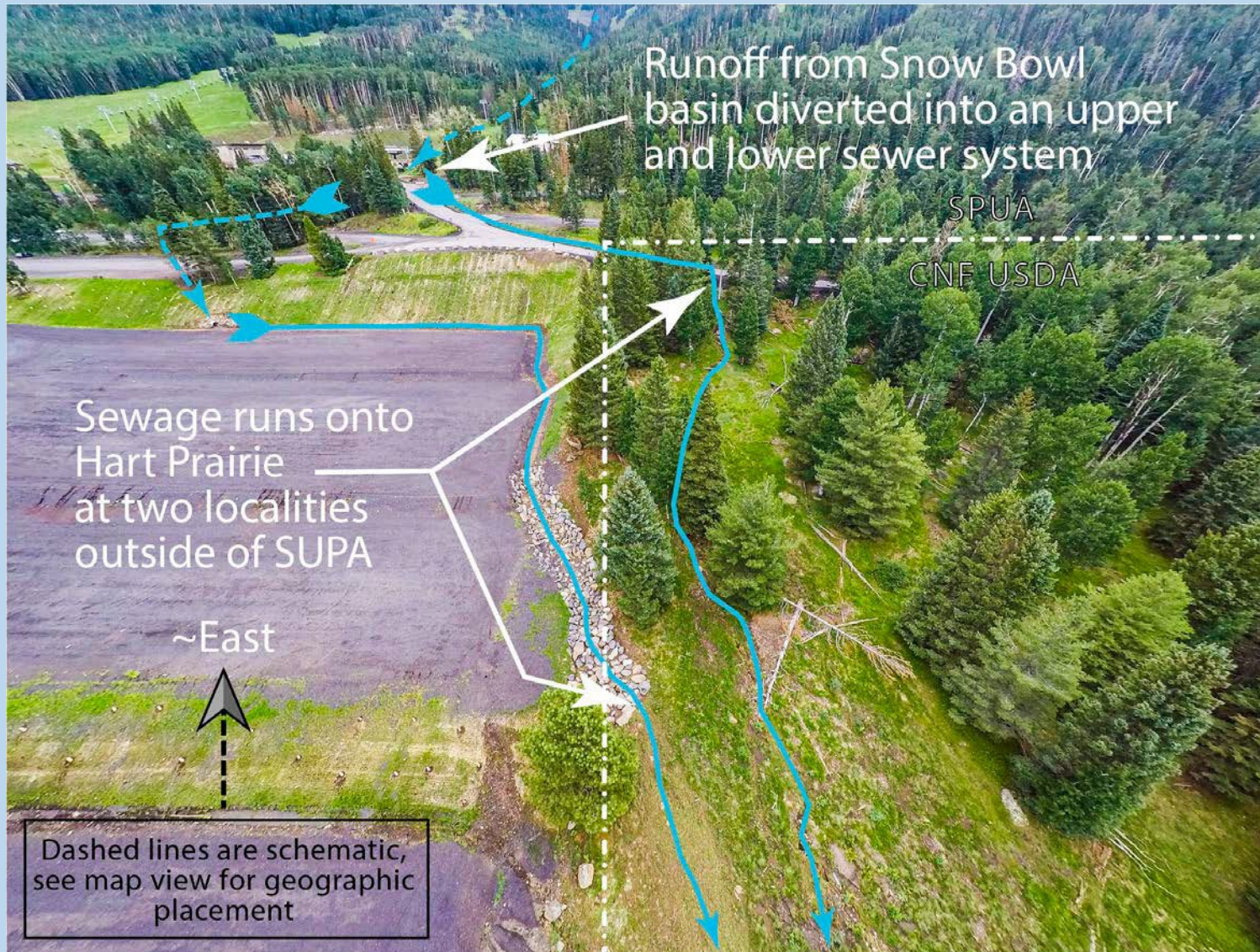
Oblique (distorted) aerial view of the terminal portion of the stormwater drainage system where it debouches onto Hart Prairie.
